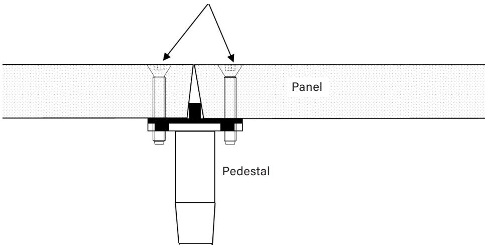
The Taptite TRILOB machine screw has a triangulated and tapered end on the screw thread so when screwed into the hole will self tap its own thread through the hole predrilled in the pedestal head.
